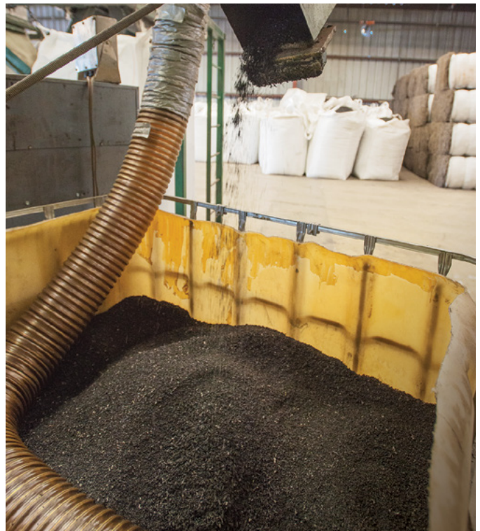
Top left: In the waste tire conversion process, old tires are sent through through an initial shredding machine where the rubber is split into big chunks. Bottom left: Multiple shredding machines work in tandem to reduce the rubber into smaller and smaller pieces. Right: The finely shredded product, now in particle form, is ready to be shipped in super sacks, background. Caltrans diverted about 4.6 million tires from landfills in 2015.
