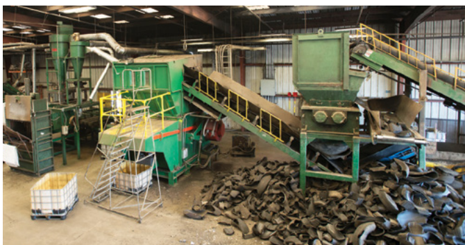
Top left: In the waste tire conversion process, old tires are sent through through an initial shredding machine where the rubber is split into big chunks. Bottom left: Multiple shredding machines work in tandem to reduce the rubber into smaller and smaller pieces. Right: The finely shredded product, now in particle form, is ready to be shipped in super sacks, background. Caltrans diverted about 4.6 million tires from landfills in 2015.
